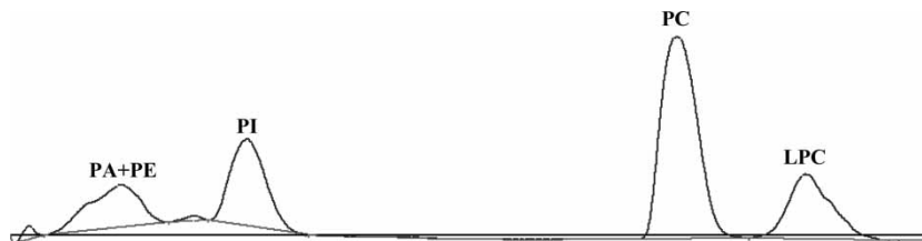
Figure 10. TLC-FID chromatogram of a commercial lecithin type II (PA = phosphatidic acid, PE = phosphatidylethanolamine, PI = phosphatidylinositol, PC = phosphatidylcholine, LPC = lysophosphatidylcholine).
